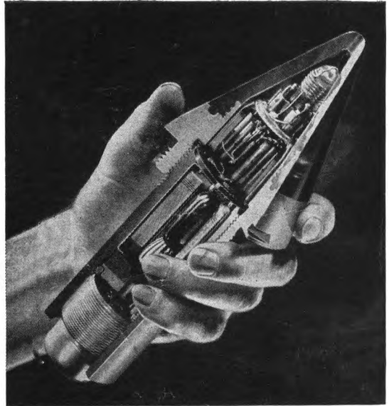
FIVE-TUBE RADIO transmitter and receiver, in the nose of the shell, is the heart of the secret weapon. In flight, the transmitter broadcasts a continuous radio wave. Reflected back from the target, this wave explodes the shell at exactly the right moment!
